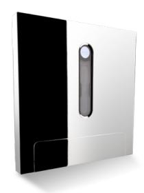
signals for the RF remote and upcoming Wi-Fi option (explained below) to enter the chassis. At the front of that strip is a circular display that indicates the volume level, input selected, and phase setting. If you hold the Source button down for a few seconds, the incoming sample rate is displayed. All told, the D-Premier is one of the most elegant-looking pieces of hi-fi gear to come my way in a long time. It's a work of industrial art.
